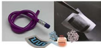
Flexible toy pencils deposit a polymer/graphite composite to make a chemical vapor sensor. Figure courtesy of Jiaxing Huang. Click image to enlarge.
